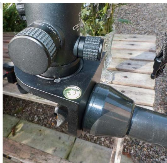
**\*\* Important\*\*** both the male and female screw threads are 3/8" and so you must make sure that both your tripod - and tripod head - can accommodate this larger size thread. Fortunately the Benbo has a 3/8" thread at one end and a 1/4" thread at the other - and the Giottos MH1302-652 series 2 ball head has a 1/4" adapter that can be removed to reveal a 3/8" screw thread. Check before you buy.
