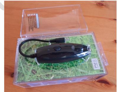
Once removed you can again feel the quality of its sturdy construction. This isn't something that is going to get damaged easily. This is version 2 of the Powermonkey and has a sliding on/off switch and recessed LED lights.
