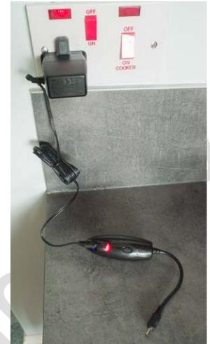
It took approximately 1 hour to charge which, based on the quoted charging time for the mains charger vindicates the '60% charged on arrival' claim.
