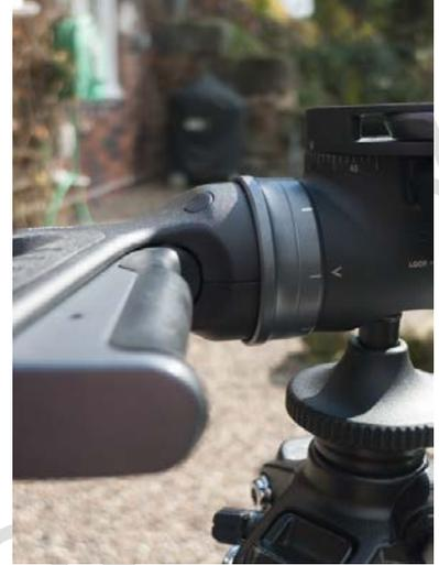
Removal of the camera & top-plate is easy. Just press the orange safety catch and flick the silver lever.
