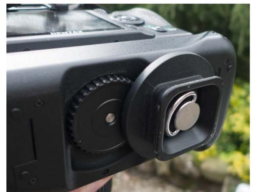
A spigot automatically locks the plate onto the pistol grip as soon as it is fitted. The top of the grip also has a useful spirit level for alignment before taking panoramas (more on that later).
