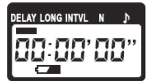
With any remote cable release, if the camera is set to bulb setting then the release button can be locked - very useful for long-exposure shots when the shutter release time is critical (when using a 9-or-10 stop neutral density filter, for example). This unit goes one better - as soon as the shutter release is locked down it starts the timer so you can see exactly how long the exposure has been. Beats a separate watch or timer, for sure.
